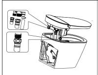
(1) connect and tight the three braided hoses to E-bidet by wrench, then insert the hose and install the clamp.
