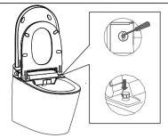
(3) Place the gasket on both sides of the E-bidet lock the screw and insert the rubber pads. Then turn on the water supply and plug in.
