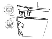
(2) Align the location hole of E-bidet with toilet bowl guide pillar, press into the electronic cover .
